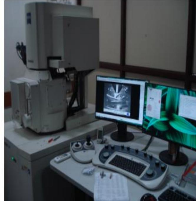
Field Emission Scanning Electron microscope (FESEM)
