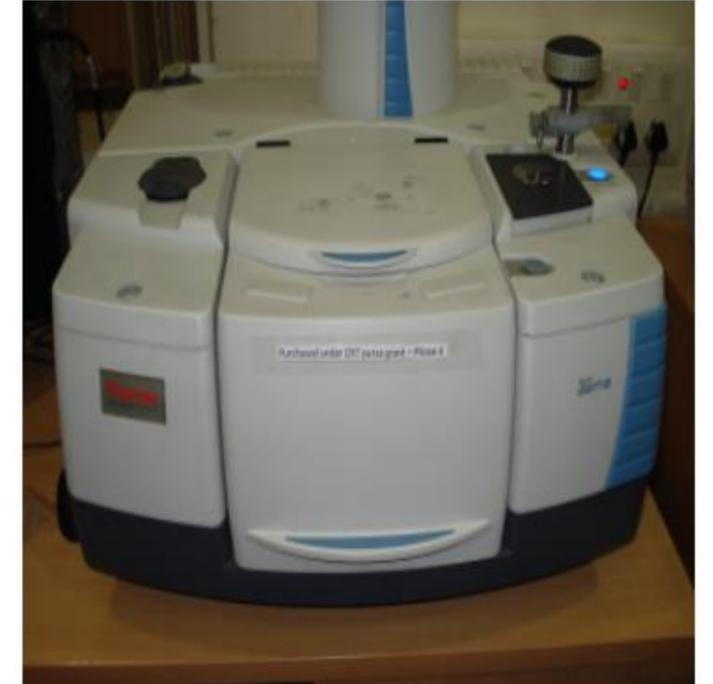
Fourier-Transform Infrared Spectroscopy (FTIR)
